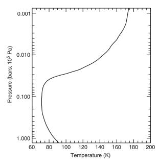
**Figure 17** Temperature versus pressure on Titan as obtained by Voyager radio occultation.
